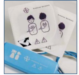
Pads are non-polarized and can be placed in either the chest or back position.
